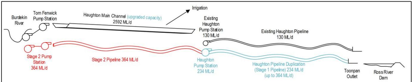
Option 2 provides for supply of 364 ML per day. In the first 15 years, this would be supplied through the upgraded channel. After 15 years, 364 ML per day could be supplied through the pipeline. The capacity left in the channel could then be used by irrigators. As Stage 1 has a capacity of 364 ML per day, the construction of the Stage 2 pipeline does not provide additional capacity when compared with the upgraded Sunwater channel.
