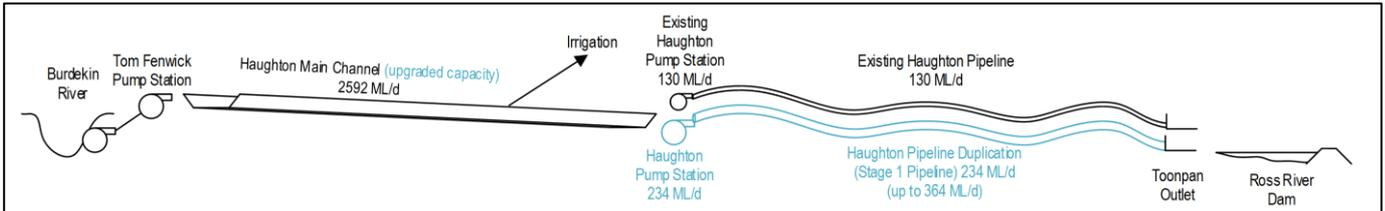
Initially, under Stage 1, the Haughton pump station will be able to pump 234 ML per day, in addition to the 130 ML per day that can be pumped through the existing pipeline. However, when the existing pipeline is decommissioned, the Haughton pump station will be upgraded to allow 364 ML per day to be pumped through the new Stage 1 pipeline. Whenever the council is not using the Sunwater channel capacity, this is generally made available to irrigators.
