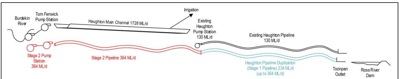
Constructing a Stage 2 pipeline now avoids the need to upgrade the Sunwater channel and the Haughton pump station—a total saving of approximately \$55 million. Under Option 1, like in the base case, 364 ML per day can be delivered.
